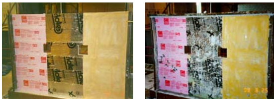
Figure 7: Cavity Wall, 2 Week Moisture Test
