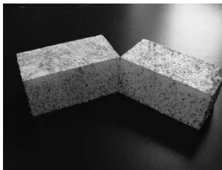
3. Expanded (EPS) with food color tracing paths of water intrusion
