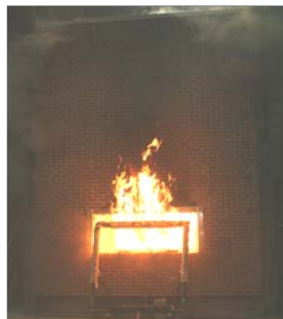
Figure 4: Fire emitting from the test window
