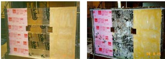
The test specimen consisted of a 12' wide by 8' high standard masonry cavity wall with three types of 2" thick insulation, extruded polystyrene (Figure 7, left sample), foil faced polyisocyanurate (center sample), and spray polyurethane (right sample).
